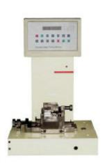
LCT plastic tensile impact testing machine is used to execute tensile-impact test of plastics or insulaton materials under defined condition, as tensile tests at relatively high strain rates; measure the tensile-impact strength and permanent break elongation rate, especially for materials too flexible or too thin to be tested use Charpy or Izod impact tester.
